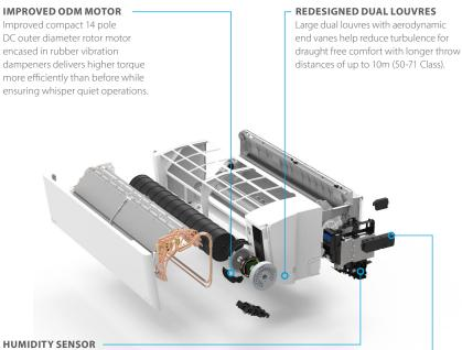
Monitors humidity to accurately control supply air temperature for comfortable and effective dehumidification of the room during Program Dry Function operation.
